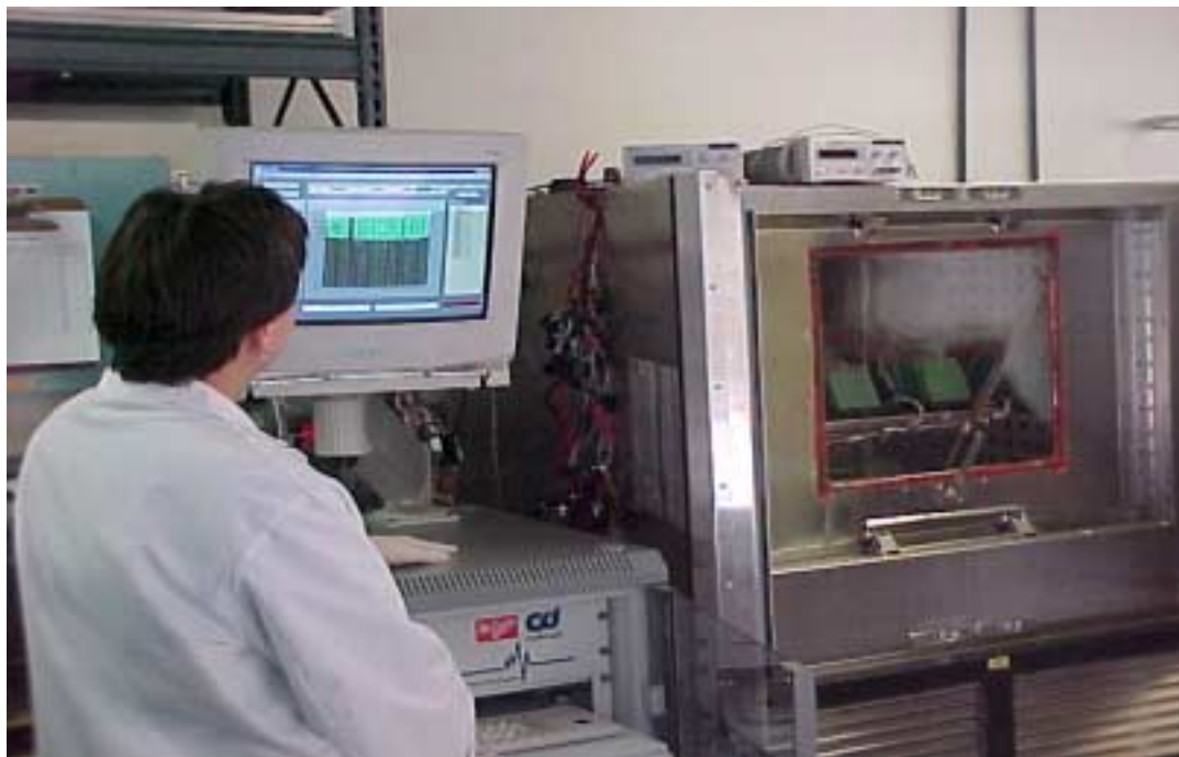
Moisture and Insulation Resistance Testing
