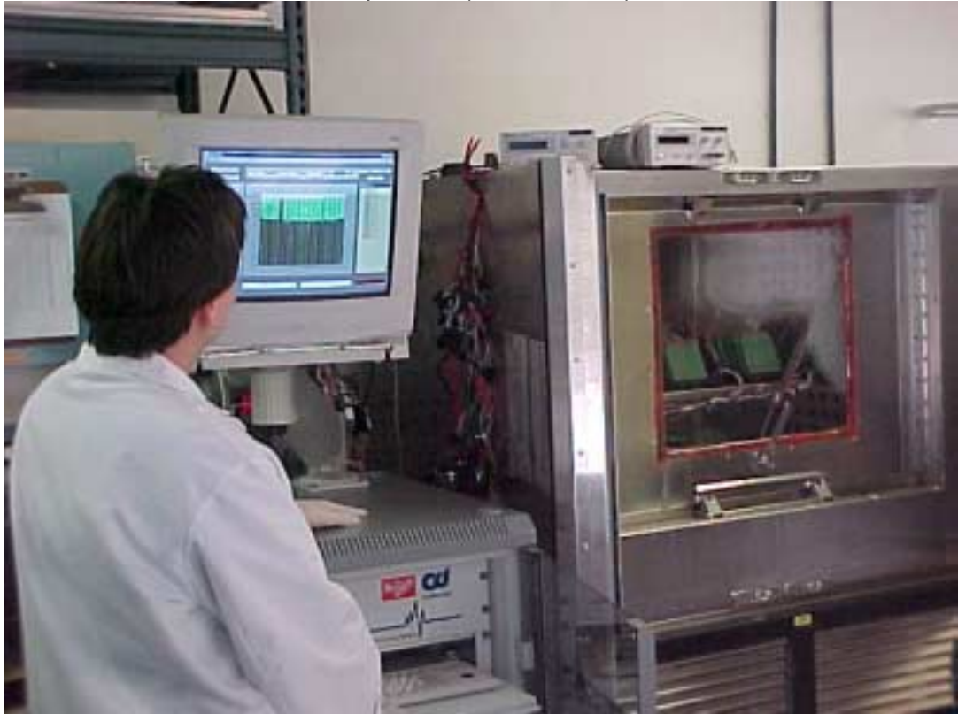
Moisture and Insulation Resistance Testing
